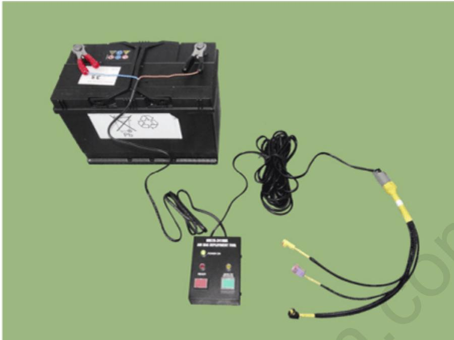
6. Activate the switch of the airbag deployment tool to deploy the airbag system.
