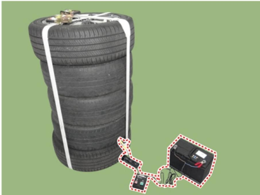
7. When the POWER ON (A) is illuminated on the airbag deployment tool, press READY (B), and then DEPLOY (C) to deploy the airbag.
